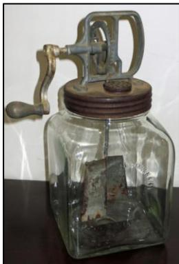
In the old days, butter was made by hand, in something called a **churn**. This churn is made of a bottle, with a lid. The lid has paddles attached inside, and a handle at
